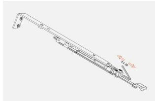
When the handle side slightly hangs down under the action of gravity, it may keep the sash at an opening status. You may adjust the bolts hidden inside the controller on the diagonal stay with hex wrench clockwise or anticlockwise to keep the sash level so that you can open it easily.
